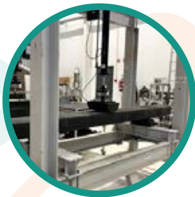
INITIAL TEST OF SLEEPER FOR RAILWAY INFRASTRUCTURE MADE OF PLASTIC.
